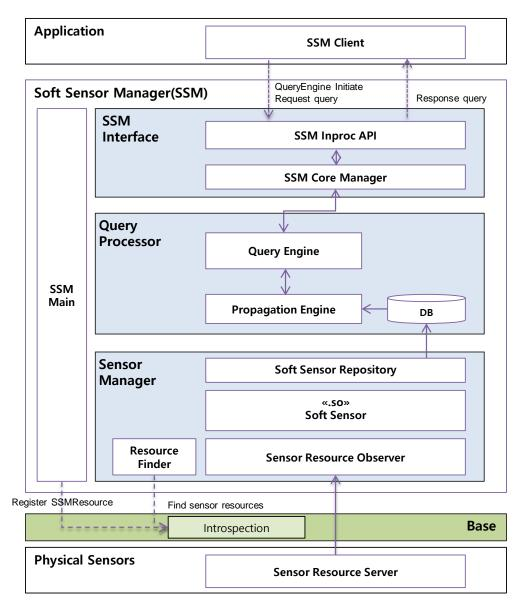
Figure 3. SSM Architecture
