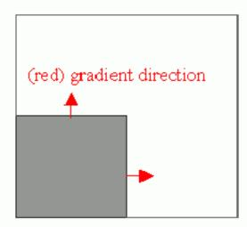
Sub-pixel accurate corner locator is based on the observation that every vector from the center q to a point p located within a neighborhood of q is orthogonal to the image gradient at p subject to image and measurement noise. Consider the expression:
