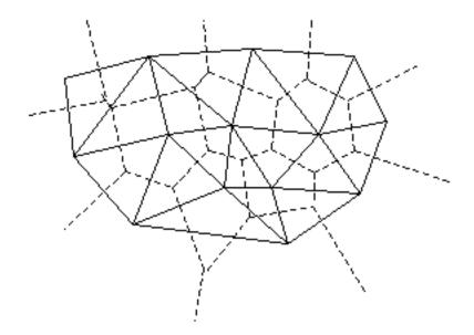
OpenCV subdivides a plane into triangles using the Delaunay's algorithm. Subdivision is built iteratively starting from a dummy triangle that includes all the subdivision points for sure. In this case, the dual subdivision is a Voronoi diagram of the input 2D point set. The subdivisions can be used for the 3D piece-wise transformation of a plane, morphing, fast location of points on the plane, building special graphs (such as NNG,RNG), and so forth.
