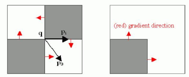
Sub-pixel accurate corner locator is based on the observation that every vector from the center q to a point p located within a neighborhood of q is orthogonal to the image gradient at p subject to image and measurement noise. Consider the expression:
