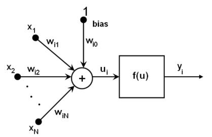
In other words, given the outputs  $x_i$  of the layer n , the outputs  $y_i$  of the layer n + 1 are computed as:
