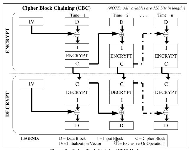
Figure 2: Cipher Block Chaining (CBC) Mode
