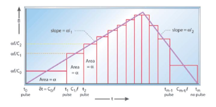
This implies the the width of the pulses must decrease as the motor accelerates. That is the pulse with has to be computed while the motor is in motion. This is illustrated in the above drawing. A program to accomplish this might look something like the following:
