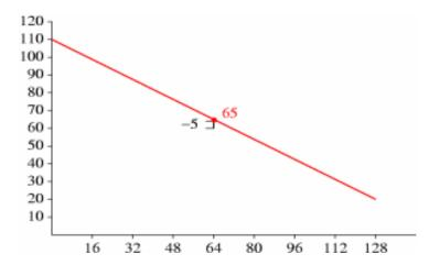
We now draw new logical lines to reflect the correction to new\_Y, and iterate for X positions 32 and 96:
