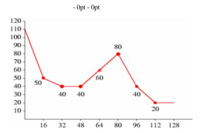
A more efficient algorithm with carefully defined integer rounding behavior is used for actual decode, as described later. The actual algorithm splits Y value computation and line plotting into two steps with modifications to the above algorithm to eliminate noise accumulation through integer roundoff/truncation.
