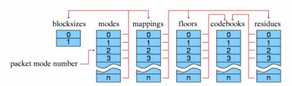
The setup header contains the bulk of the codec setup information needed for decode. The setup header contains, in order, the lists of codebook configurations, time-domain transform configurations (placeholders in Vorbis I), floor configurations, residue configurations, channel mapping configurations and mode configurations. It finishes with a framing bit of '1'. Header decode proceeds in the following order:
